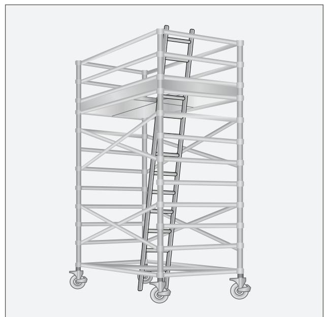
Figure 5 Mobile scaffold with an access ladder and a trapdoor to provide the largest possible hazard-free working platform.
